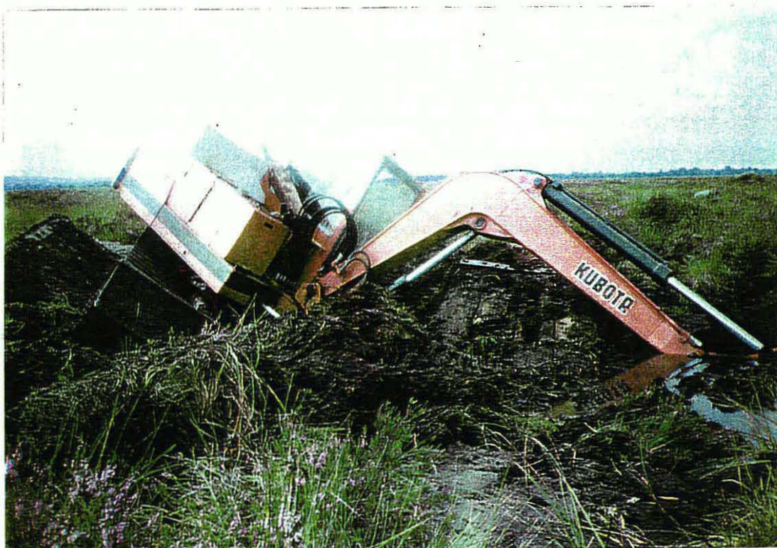
Plate 6. Machine sank due to inadequate mats and very wet conditions. August 96'
