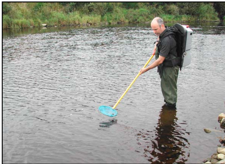
Plate 2 Semi-quantitative electrical fishing on sub-optimal habitat.
