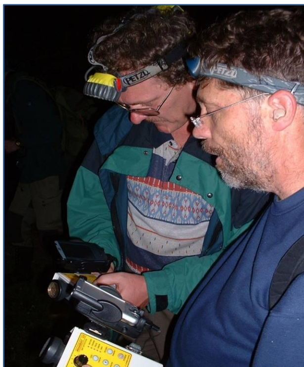
Figure 10 Using heterodyne and time-expansion bat detectors in the field. [Photograph: Conor Kelleher]
