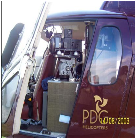
Plate 2. Position of thermal-imager in helicopter.
