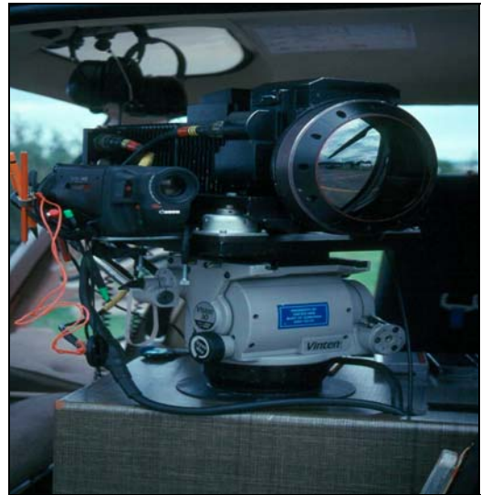
Plate 3. Thermal-imager mounted on pan & tilt head.
