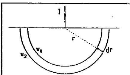
Figure 4. Point electrodes on the surface of a homogeneous earth.
