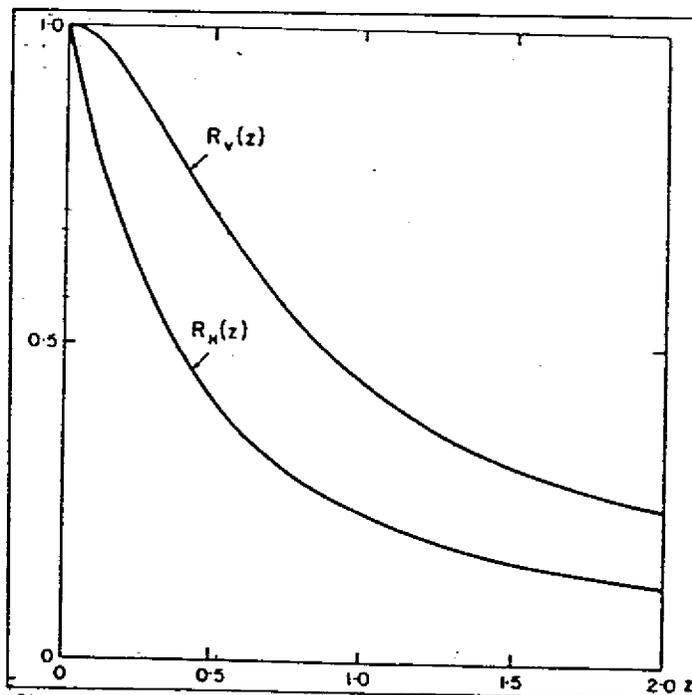
Figure 10. Cumulative response versus depth for vertical and horizontal dipoles. (McNeill, 1980).
