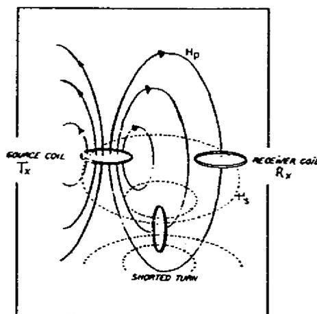
Figure 7. The basic principle of the electromagnetic method.
