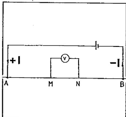
Figure 5. The potential V between M and N is caused by influx of current + I at point A and an outflux of current - I at point B.
