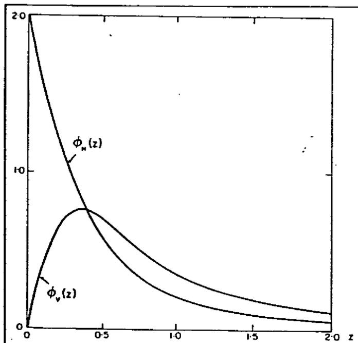
Figure 9. Comparison of relative responses for vertical and horizontal dipoles. (McNeill, 1980).
