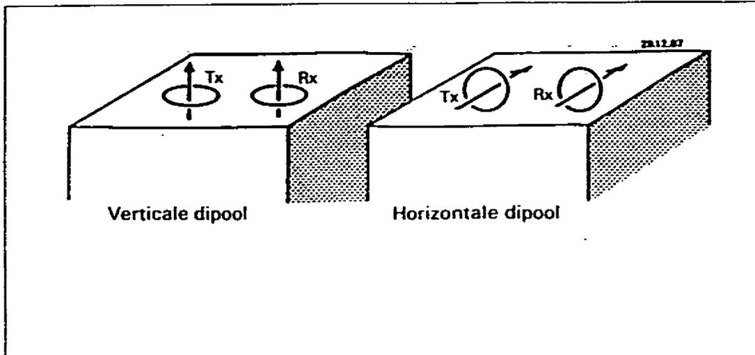
Figure 8. Vertical and horizontal dipole configuration (Biewinga, 1990/1991).
