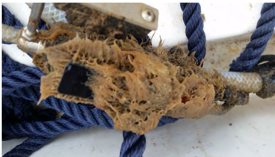
Figure 9-20 Biofouling on the top turbidity sensor on Buoy 2 in July 2020
