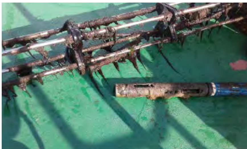
Figure 9-9 Fouling of East Link sonde after 3 weeks deployment in August 2019
