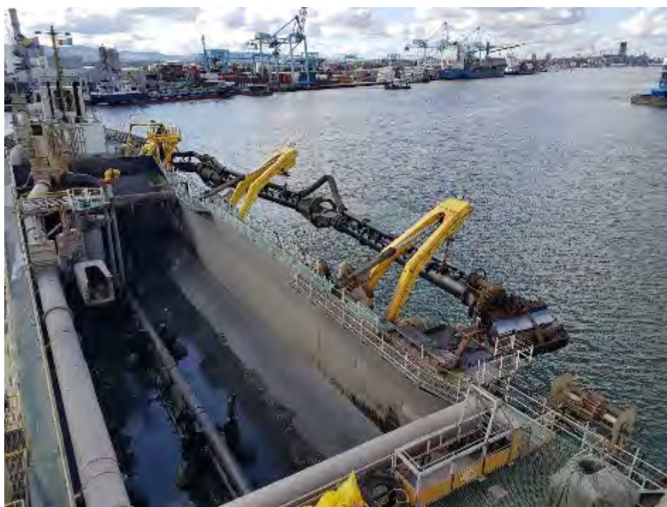
Plate 3-11 Typical Trailing Suction Hopper Dredger Arrangement
