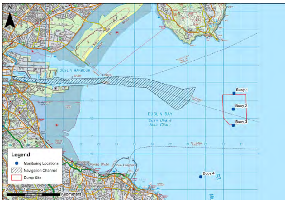
Figure 9-19 Locations of the Coasteye buoys at the dump site (buoys 1 to 3) and background site (buoy 4) Turbidity and Total Suspended Solids
