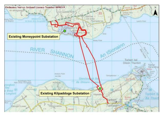
Figure 1 Project location map Foreshore Licence Area (98.15 ha) is highlighted in red which also shows the proposed submarine cable corridor.
