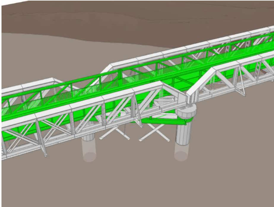
Figure 4. New Truss Typical Section & 3D Model View
