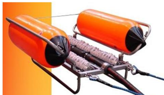
Figure 2-5: Example of Sparker Sub-Bottom Profiler
