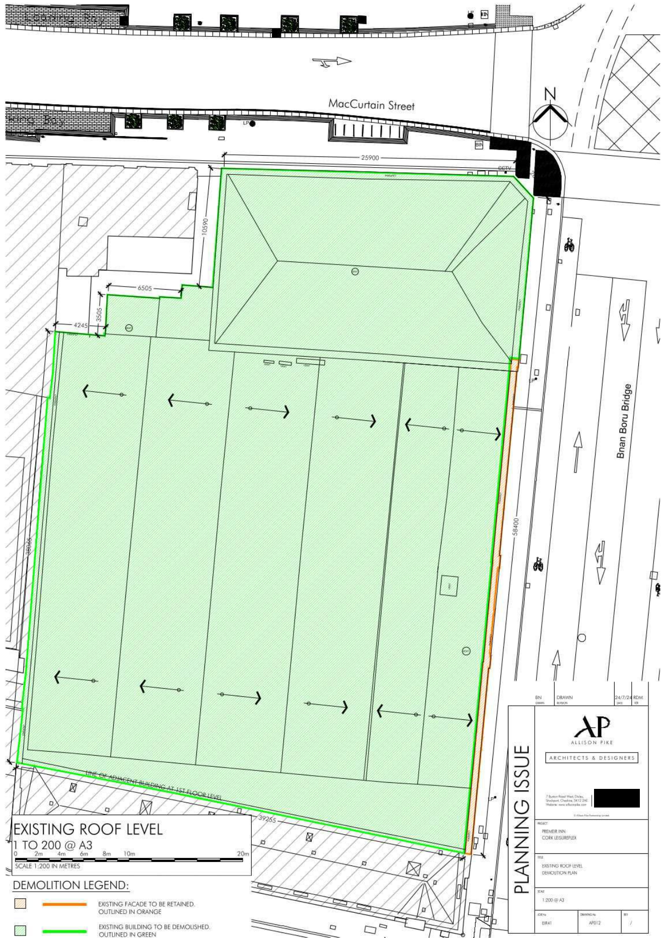
Figure 2. Demolition plan (roof level)
