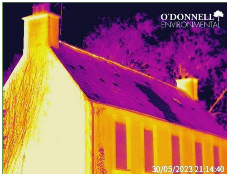
Plate 2.1 Example image from thermal camera covering the front/eastern aspect of Roseville House.
