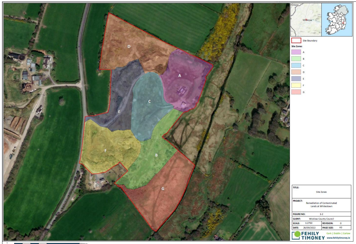
Figure 6-1: Remediation Zones (The original bat roost structures are located in zone A and the compensatory bat roost is located in zone D).
