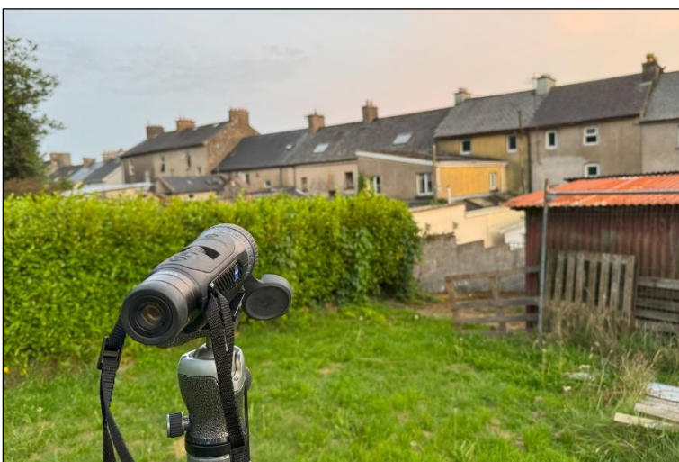
Plate 12 Vantage point survey using thermal imaging scope (Zeiss DTI6/40).
