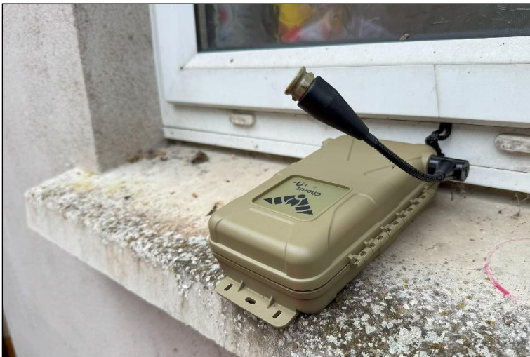
Plate 11 Anabat Chorus unit installed at the subject site.
