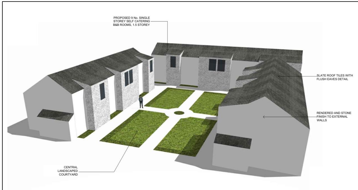
Figure 2-1. Concept 3D view of units to rear of subject building (Demesne Architects + Interior Designers).
