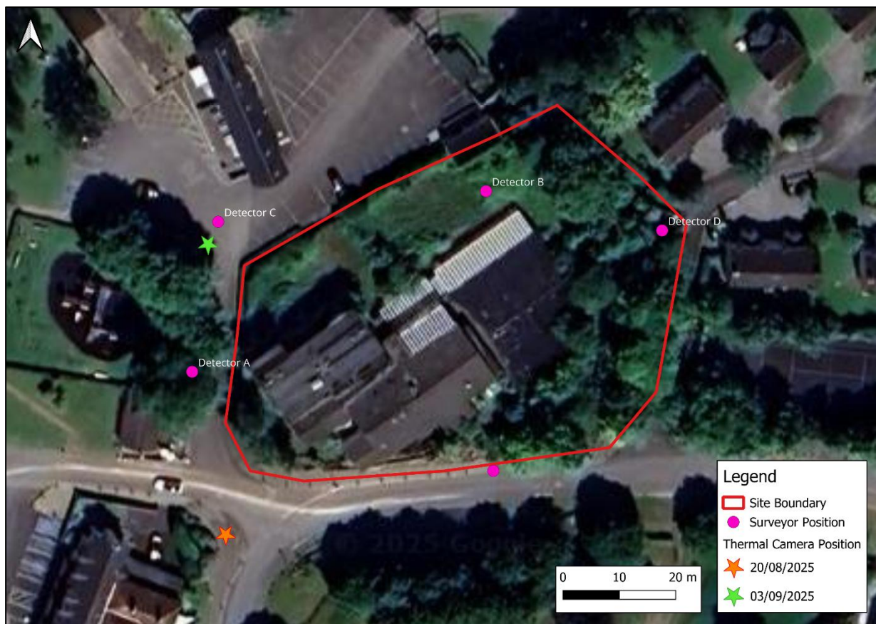
Figure 4 shows the location of surveyors and thermal camera during both emergence surveys.
