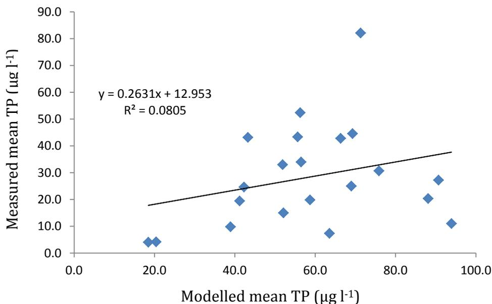
**Figure 11.10** The relationship between the modelled and measured TP based on the full model with the higher livestock P inputs, and excluding Ballindereen.
