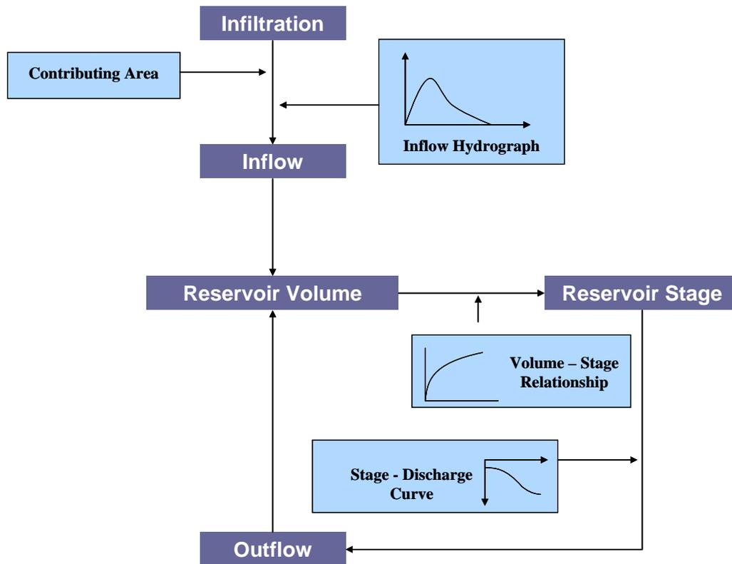
Figure 3.81 Flow chart for reservoir modelling methodology
