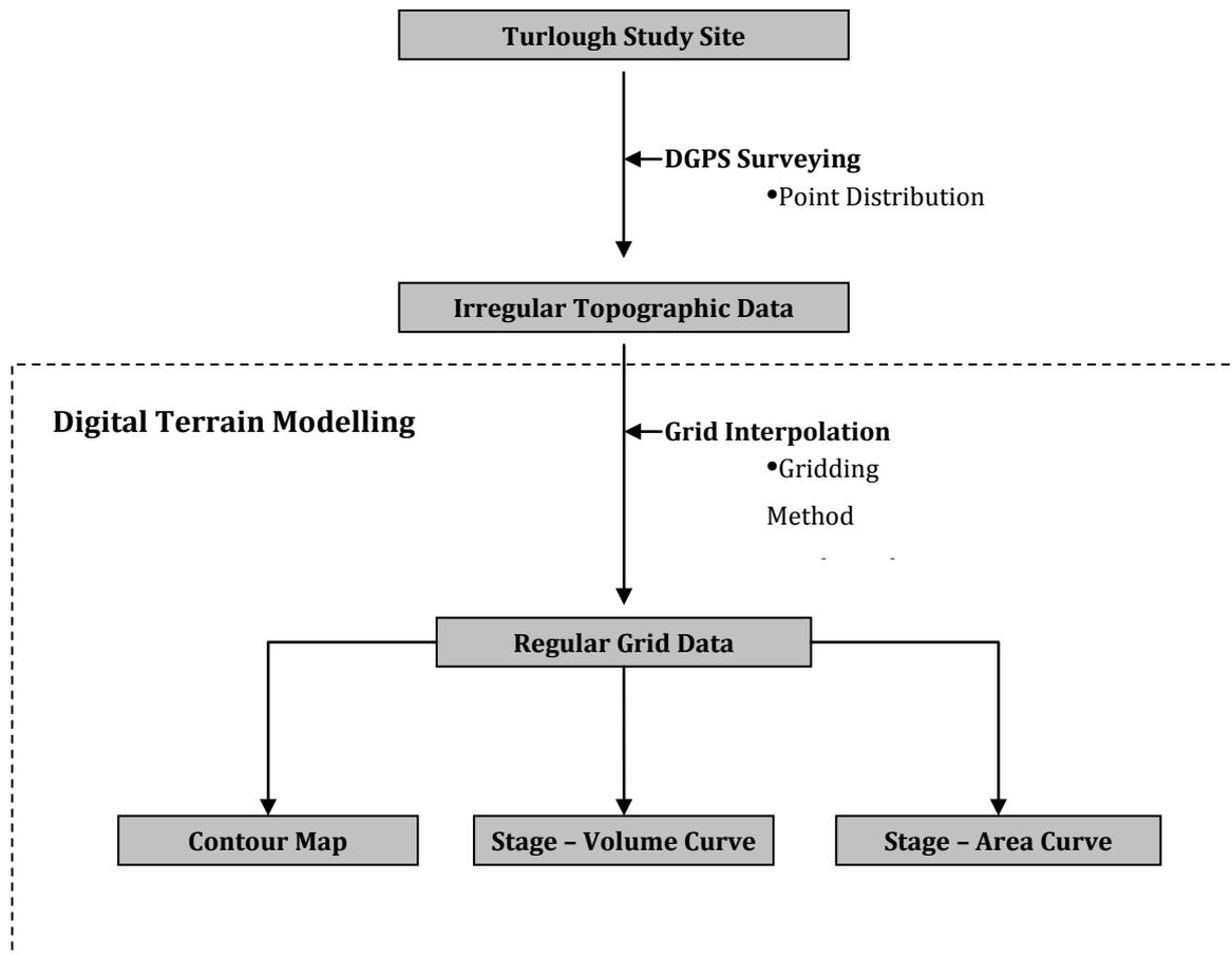
**Figure 12.2.** Flow diagram of the steps required to develop ecologically relevant hydrological variables from dGPS survey and water level data.
