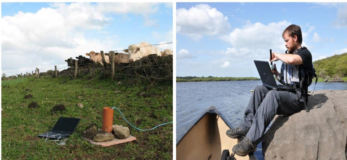
**Figure 12.1.** Diver platform, Rathnalulleagh, Co. Roscommon (left), and downloading diver using Reading Unit, Garryland, Co. Galway (right)
