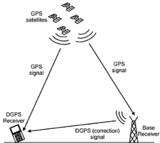
**Figure 3.9** Conceptual operation of differential GPS surveying system (from Maini & Agrawal, 2007)
