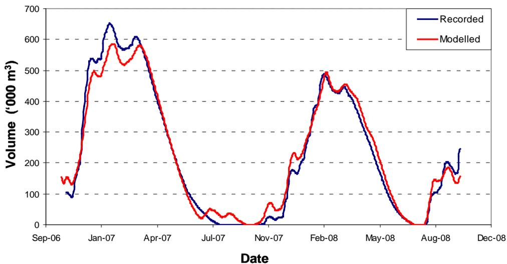
**Figure 3.94** Plot of recorded and modelled volume for Ardkill, Co. Mayo
