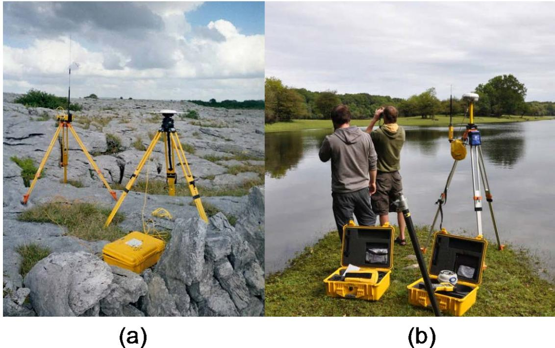
**Figure 3.10** Trimble 4700 GPS system (a) and Trimble R6 GPS system (b)
