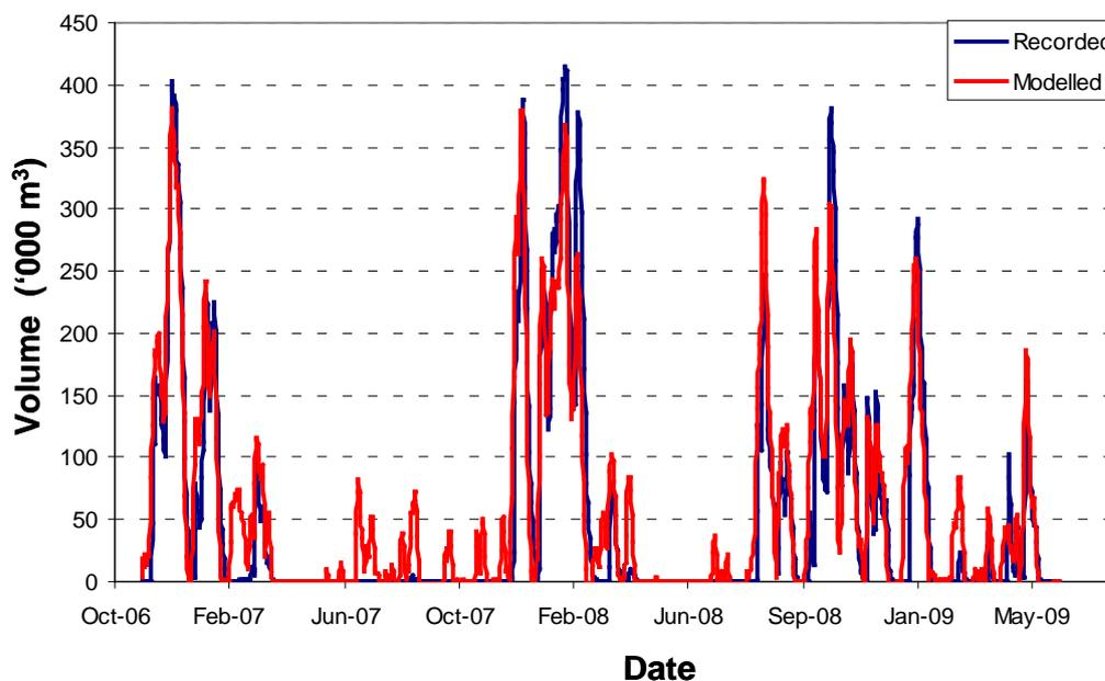
Figure 3.92 Plot of recorded and modelled volume for Turloughmore, Co. Clare
