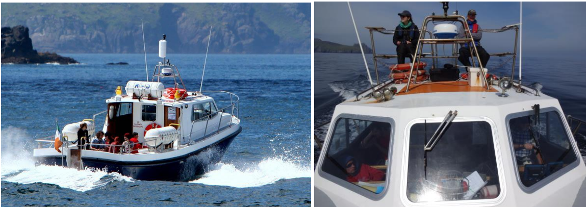
Fig. 2. MV An Blascaod Mór with flying bridge suitable for line-transects
